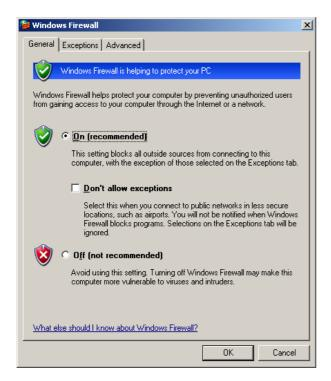
Select the "Exception" tab and add SpectraLiveClient.exe to the exception list. Also check if Microsoft Management Console (used by DCOM configuration utility in the next section) is in the list. If not, just add also this application.
