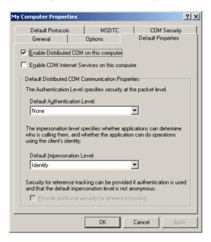
Go to COM Security tab and note these are four permission configurations. Three of these we will have to edit:
