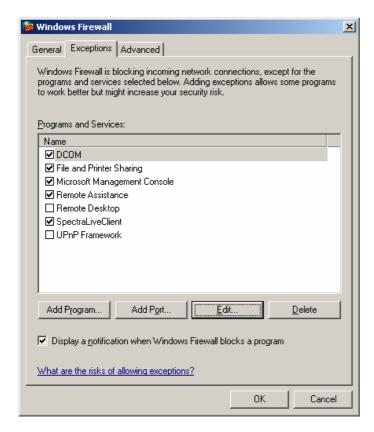
Add TCP port 135 at it is needed to initiate DCOM communication, and allow for incoming echo requests. In the Exception tab of the Windows Firewall, click on Add Port
